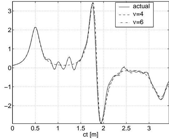
Figure 4: Pulse reflection from a heterogeneous laminate with a thin fault  $d_f = 2^{-7}$  and  $\varepsilon_f = 20$ , at  $z_f = 0.5$ . Note the doublet-type pulse at  $ct = 1.9$  which is absent in the fault-free response of Fig. 1.
