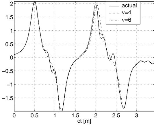
Figure 3: Pulse reflections from a heterogeneous laminate with a thick fault  $d_f = 0.5$ ,  $\varepsilon_f = 1$  at  $z_f = 0.25$ . Note the doublet-type pulse between  $ct = 1.1$  and  $2$ , which is absent in the fault-free response of Fig. 1.
