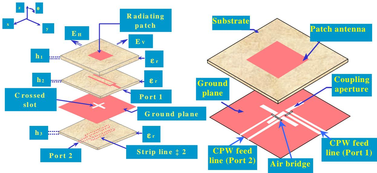
Figure 3. Polarization diversity antenna using CPW-coupled fed patch antenna with a crossed slot.
