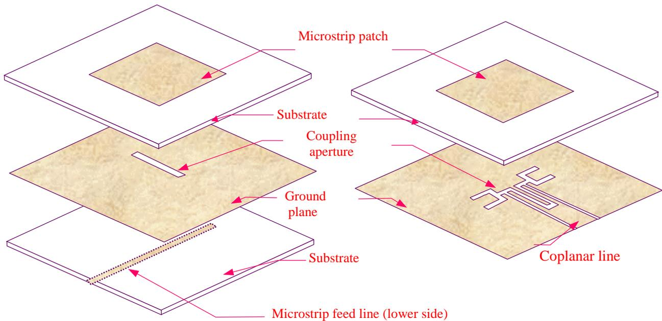
Figure 1. CPW fed patch antenna in comparison with a microstrip fed patch.
