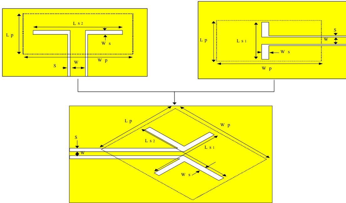
Figure 2. Dual frequency CPW fed patch antenna .
