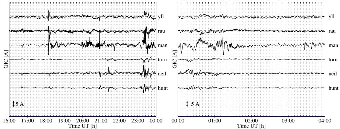
Figure 1: GIC at the Scottish and Finnish power system neutrals and at the Finnish pipeline on April 6 (left) and 7, 2000.
