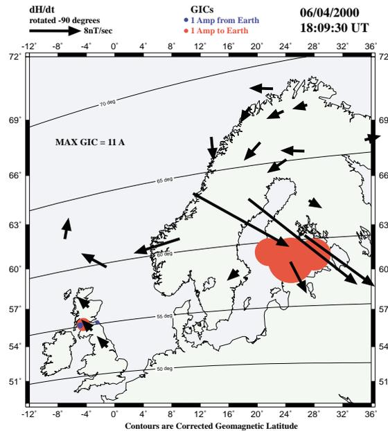
Figure 3: GIC at the Scottish and Finnish power system neutrals and at the Finnish pipeline and  $d\mathbf{H}/dt$  pattern ( $\mathbf{E}_{sur}$ ) of the geomagnetic field on ground on April 6, 2000 at 18:09 UT. Ends of arrows indicate the locations of magnetometer stations. GIC measurement locations (from west to east) are in Hunterston, Neilston, Torness (all in Scottish power system), Rauma (Finnish power system), Mäntsälä (Finnish pipeline) and Yllikkälä (Finnish power system).
