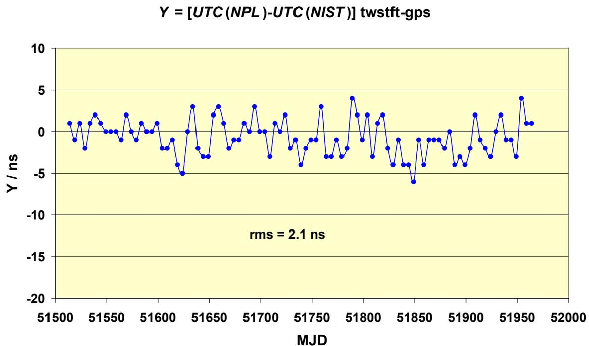
Fig. 1. Differences between TWSTFT and GPS common-view for NPL/NIST link.
