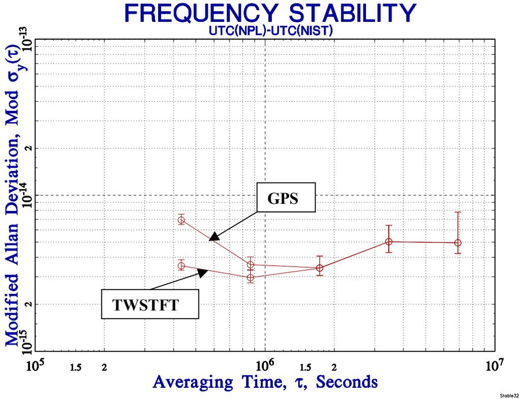
Fig. 2. Frequency stability of  $[UTC(NPL) - UTC(NIST)]$  by GPS and by TWSTFT.
