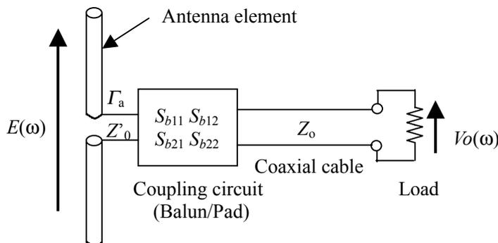
Fig.1 Dipole antenna with a coupling circuit
