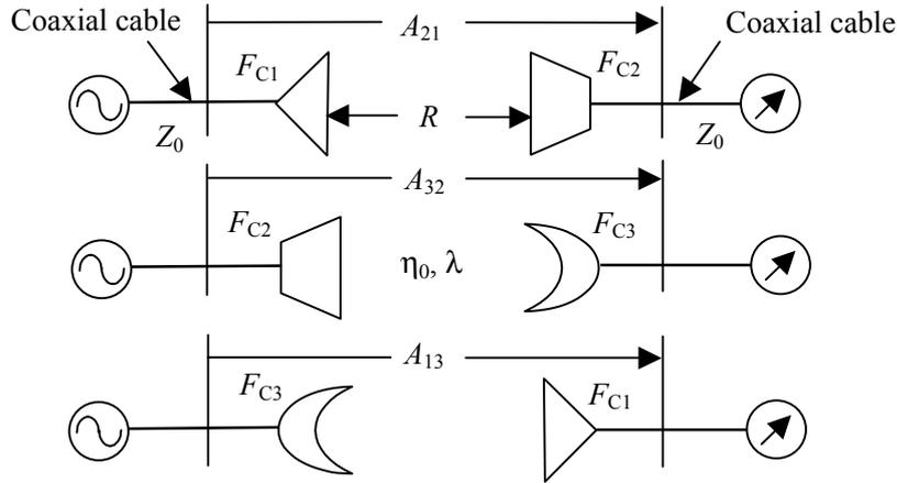
Fig.2 Three antenna method
