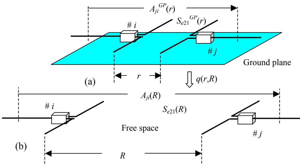
Fig.3 Measurement of transmission S-parameter and field transfer factor
