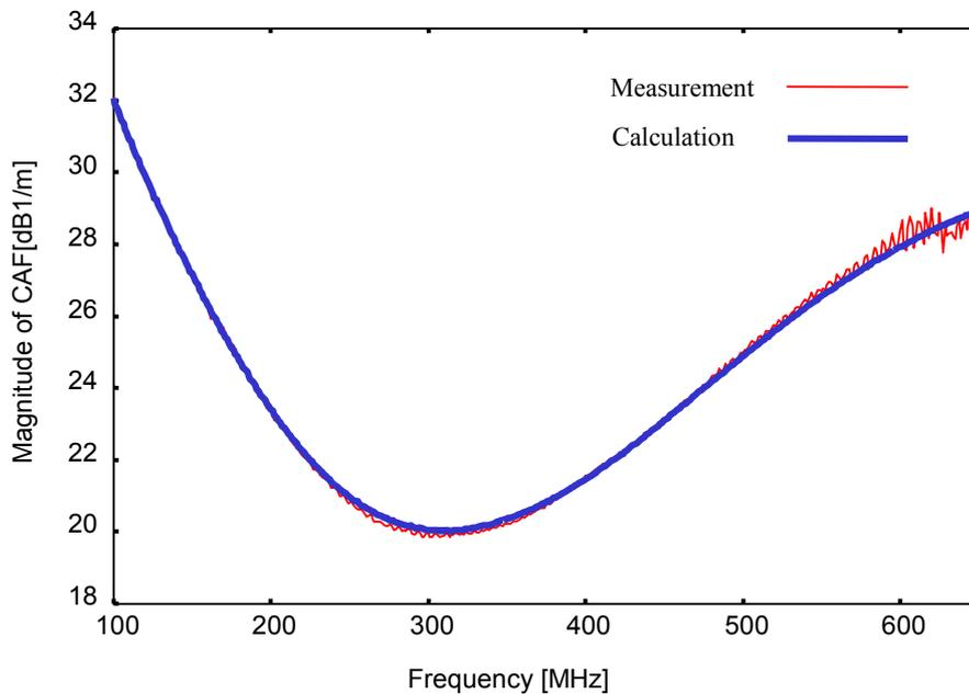
Fig.4 Measured and calculated CAF magnitude
