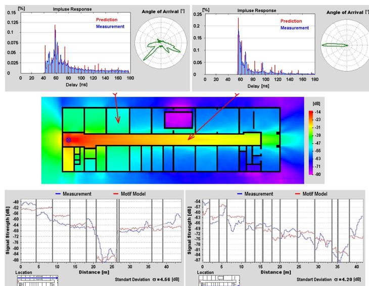
Fig. 2. Sample of the communication channel parameters prediction by Motif Model
