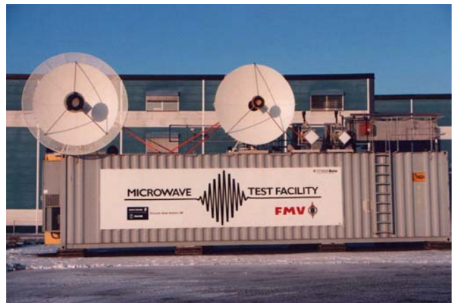
Fig. 2. Cassegrain antennas for S-band, 37 dB i (left) and C-band, 40 dB i .
