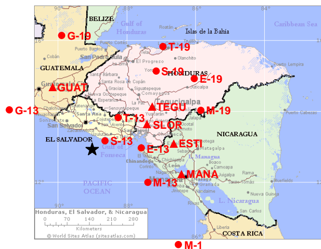
Fig. 1. The black star shows the epicenter of El Salvador Earthquake on Jan. 13, 2001. The red triangles show the operating GPS receivers and the red dots show the associated ionospheric points.
