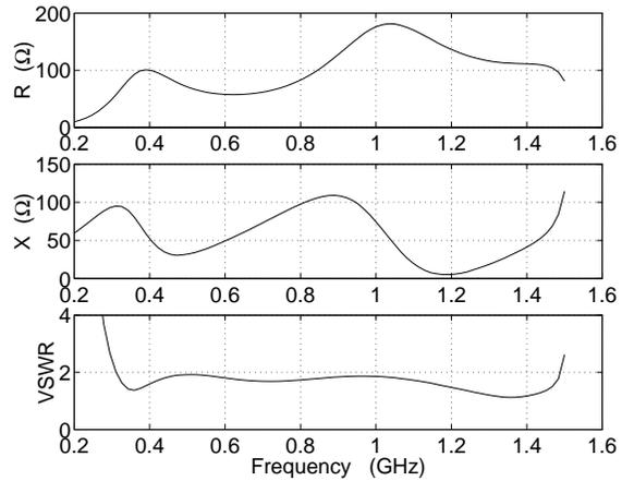
Figure 2: Infinite-array active input impedances, and standing wave ratio w.r.t.  $100 \Omega$ , after introduction of a  $4 \text{ pF}$  capacitance.
