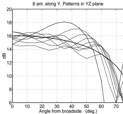
Figure 5: Element patterns for 8 antennas along  $\hat{y}$ , and an infinity along  $\hat{x}$ , at 750 MHz.
