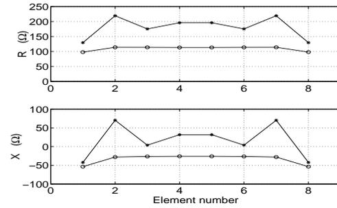
Figure 4: Active (\*) and passive (o) input impedances for an array having 8 elements along  $\hat{y}$ , scanned at broadside, at 1 GHz.
