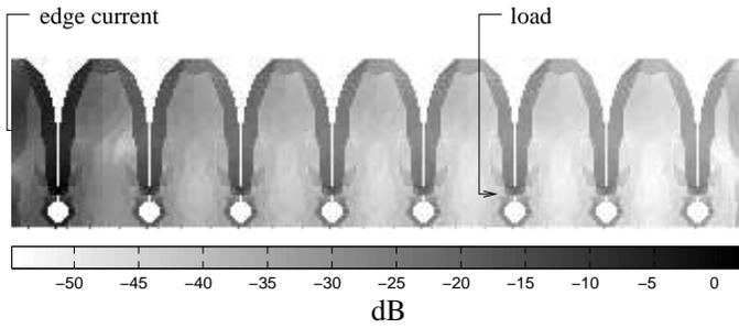
Figure 3: Magnitude of current distribution on the array infinite along  $\hat{x}$ , at 1 GHz, when the first element only is excited.
