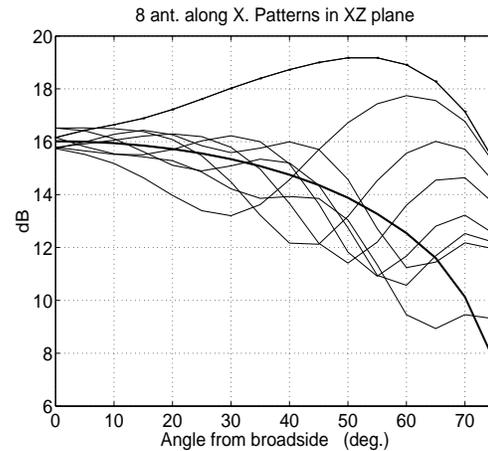
Figure 6: Element patterns for 8 antennas along  $\hat{x}$ , and an infinity along  $\hat{y}$ , at 750 MHz.
