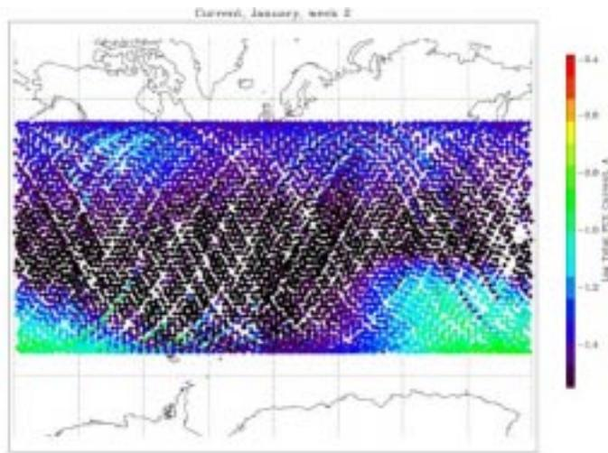
**Figure 1. The total PCU current plotted in false color along the ISS orbit on a map of the Earth**
