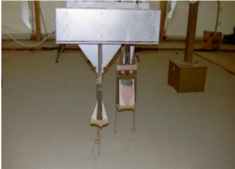
Fig. 1. Fully polarimetric GPR built in IRCTR
