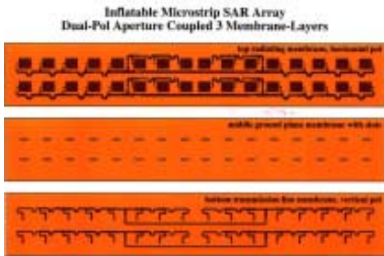
Figure 3. RF designs of the three membrane layers
