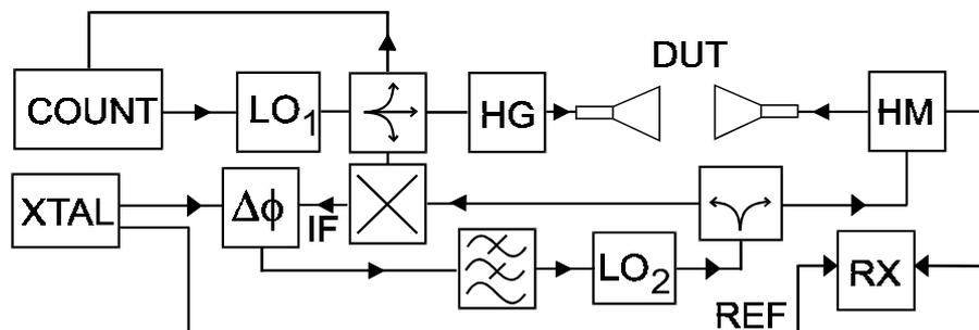
Fig.1. A schematic block diagram of the evaluated millimeter wave vector network analyzer. Two microwave sweepers ( $LO_1$  and  $LO_2$ ) are used to generate the test signal in the harmonic generator (HG) and to regenerate a lower frequency replica of it in the harmonic mixer (HM). The difference of the two local oscillator frequencies is phase-locked to a low-cost crystal unit (XTAL). Additional coarse frequency steering is provided by the external counter (COUNT) to  $LO_1$ .
