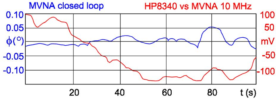
Fig. 3. Phase changes in the millimeter path (lower plot) correlate well with those of the analyzer's internal crystal reference; see e.g. the jumps at around 40 and 80 seconds. The linear drift, caused by a difference in the reference frequencies seems to be filtered out.
