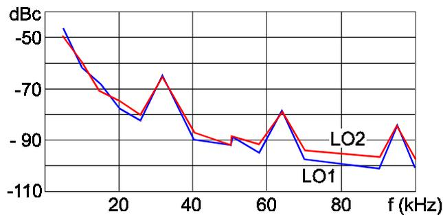
Fig. 2. The measured single-sideband phase-noise of the YIG sweepers LO<sub>1</sub> and LO<sub>2</sub> between offset frequencies of 5 kHz – 100 kHz. The measurements were done with the TEK2782 spectrum analyzer at 17 GHz (RBW=1 kHz, VBW=30 Hz, averaging=10). The added phase noise in LO<sub>2</sub> due to the PLL loop varies between 2–5 dB.
