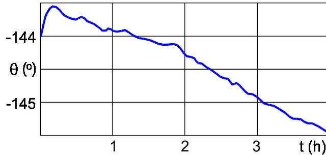
Fig. 4. Measured phase response through a straight piece of waveguide at 100 GHz during a 4 hours sampling period (after warm-up time of 24 hours). Phase drift of close to 2 degrees is observed.
