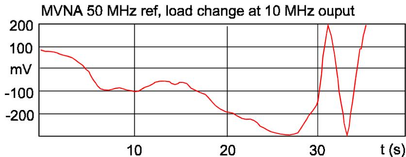
Fig. 5. One of the most primitive defects of the network analyzer's synchronization scheme is the heavy dependence of the 50 MHz reference oscillator's output frequency on the loading (changed at 30 seconds) of adjacent 10 MHz lines, which do not have a direct connection to it. Such load pulling effects seriously hamper any sensible frequency calibration efforts.
