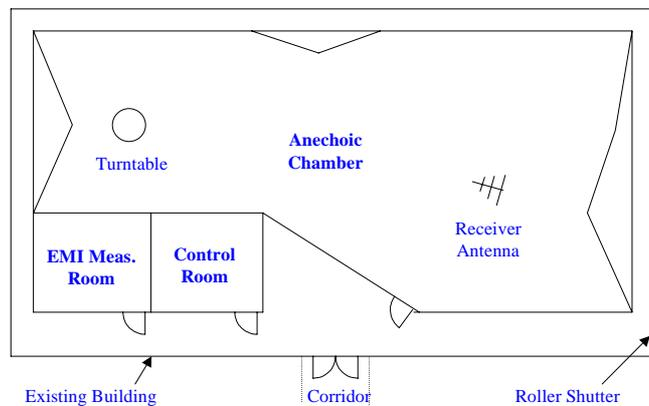
Fig. 1. Floor plan of the Asymmetrical-shaped Chamber.
