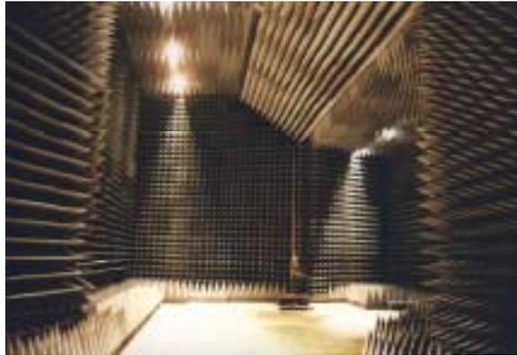
Fig. 2. Configuration of pyramidal- and wedge- shaped absorbers in the Anechoic Chamber.
