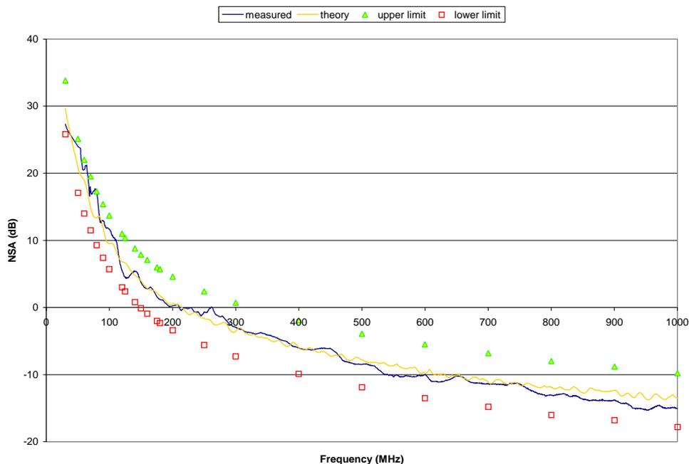
Fig. 3. Comparison between measured and calculated NSA (horizontal polarisation).
