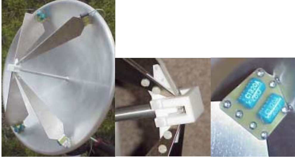
Figure 1. IRA-2 (feed arms at \pm 30^\circ ) with feed point and resistor details.
