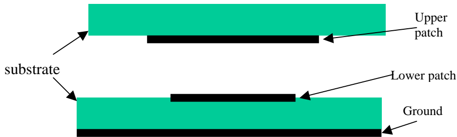
Fig. 2 Side view of the multi-layered antenna
