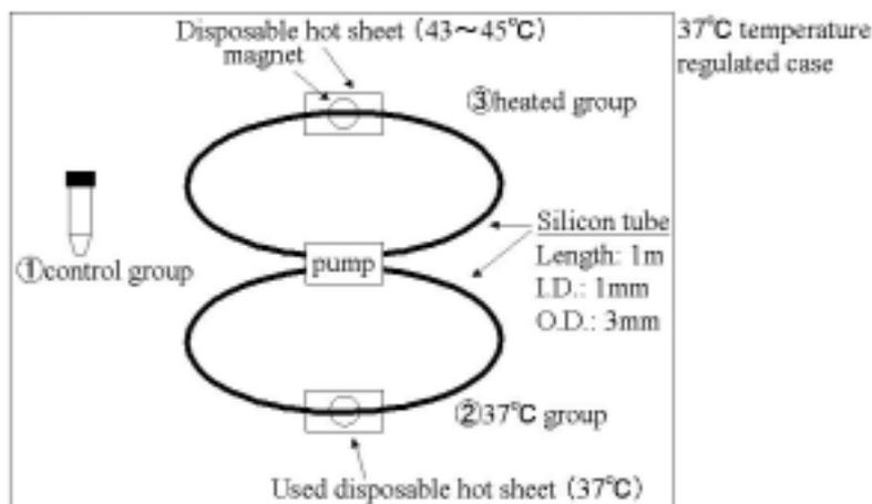
Fig. 2. Experimental system of vessel model.
