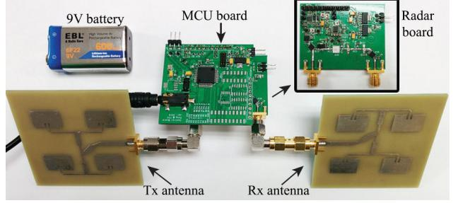
**Figure 4.** Photograph of a Doppler radar prototype (MCU: micro-controller unit, Tx: transmission, Rx: reception) [5].
