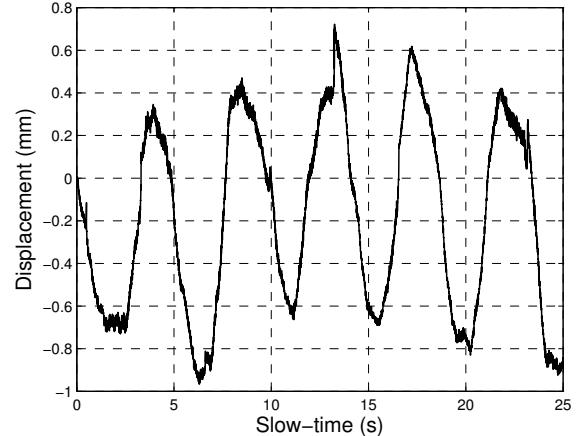
**Figure 7.** Monitored human respiration pattern obtained by the FMCW radar prototype.
