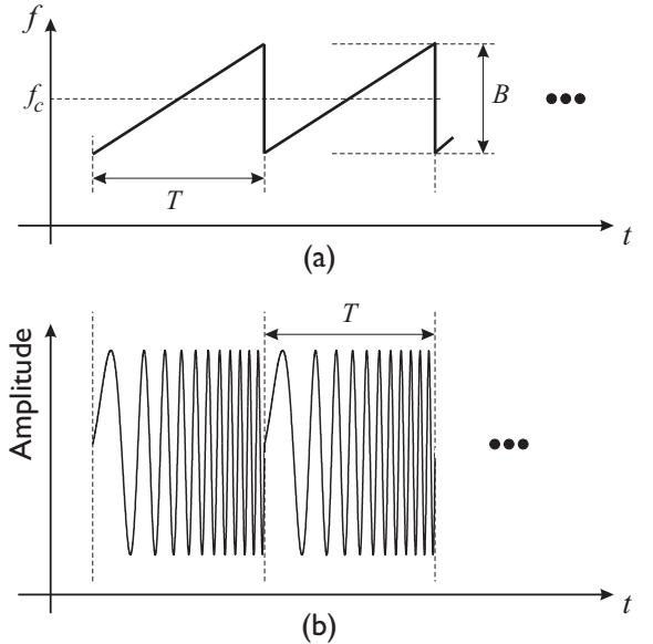
**Figure 3.** Transmitted waveform for a biomedical FMCW radar. (a) Instantaneous frequency versus time. (b) Amplitude versus time.
