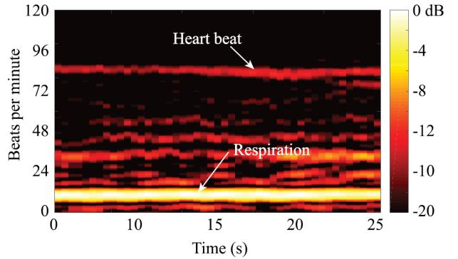
**Figure 5.** Spectrogram of vital signs extracted by the Doppler radar prototype [5].
