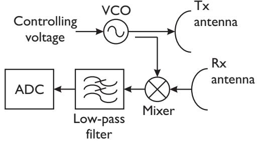
**Figure 2.** High-level schematic for a biomedical FMCW radar system (Tx: transmission, Rx: reception, VCO: voltage-controlled oscillator, ADC: analog-to-digital converter).
