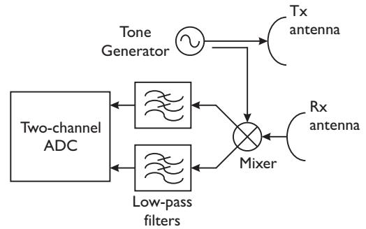
**Figure 1.** High-level schematic for a biomedical Doppler radar system (Tx: transmission, Rx: reception, ADC: analog-to-digital converter).
