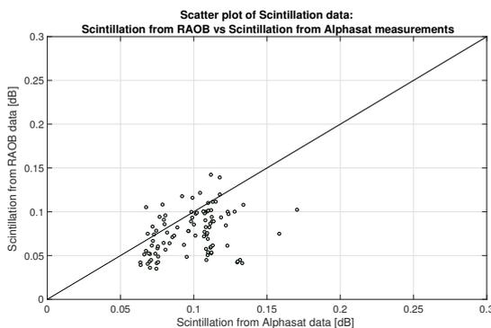
**Figure 7.** Scatter plot of Alphasat measured Scintillation vs Scintillation obtained using RAOB. August to December 2017, non rainy day)
