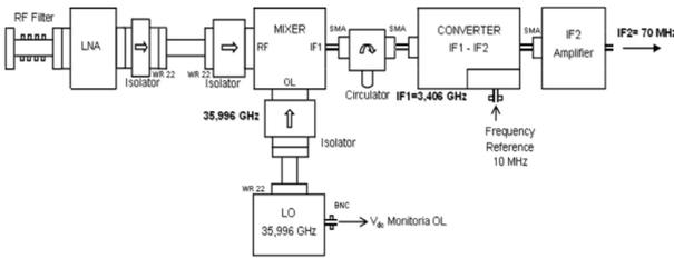
**Figure 2.** Q-band receiver block diagram.
