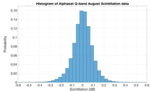
**Figure 5.** Q-band scintillation histogram of August 2017 data
