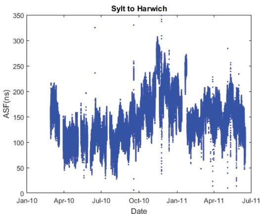
**Figure 1.** The excess propagation delay (at 100 kHz) on a 560 km all sea water between Sylt and Harwich.
