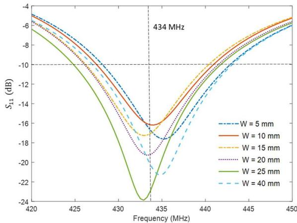
**Figure 5.** Power reflection coefficient of cavity-backed patch antenna for varying water bolus thickness.
