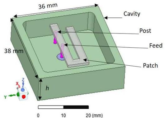
**Figure 3.** 3D numerical model of cavity backed C-patch antenna.
