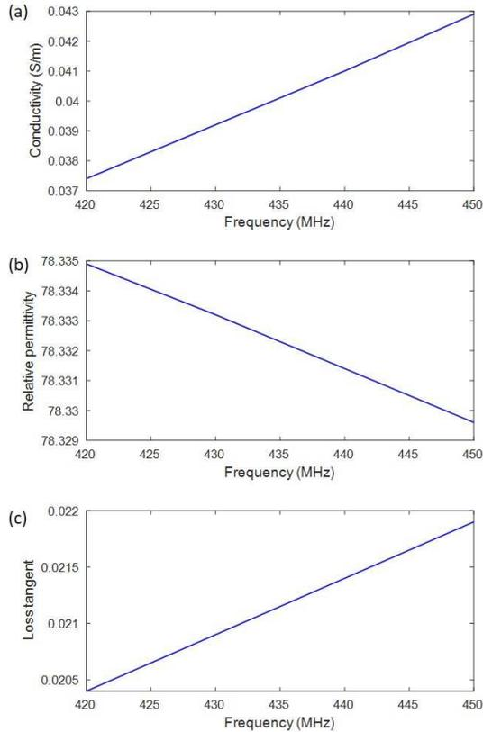
**Figure 1.** Dielectric properties (a) conductivity, (b) relative permittivity, and (c) loss tangent of DI water measure using DAK.
