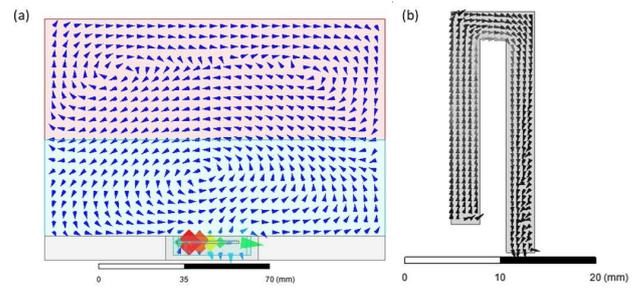
**Figure 6.** (a) E-field distribution inside water bolus and muscle phantom. (b) Current density distribution in the C-patch at 434 MHz.
