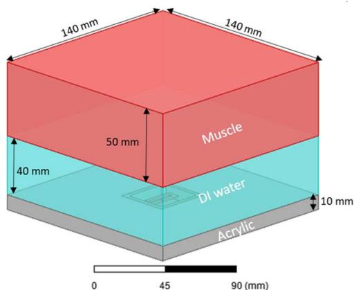
**Figure 2.** 3D model of the cavity-backed patch antenna embedded inside the acrylic sheet with water bolus and muscle phantom.
