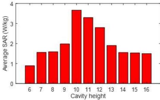
**Figure 4.** Average SAR at 5 mm depth in the tissue plane for varying cavity height.
