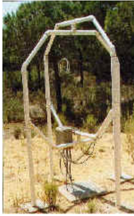
Figure: One of the seven receiving antenna of the array with North-South and East-West oriented loops which do an equilateral triangle with 62 meters of side.
