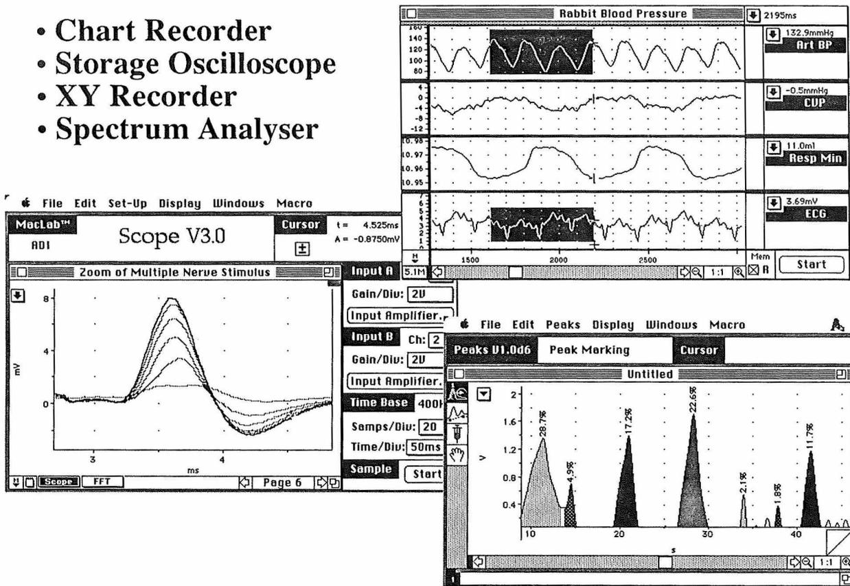
■ The range of MacLab hardware will record data on any of 4 to 8 analog channels from 1mV to 10V full scale at up to 100kHz. Additional software controlled front-end modules extend the range of the MacLab into specialist areas.
