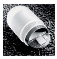
Figure 1a. The manufactured prototype of a conformal microstrip antenna by Mahe et al. [63] (©2012 Yann Mahe et al.).
