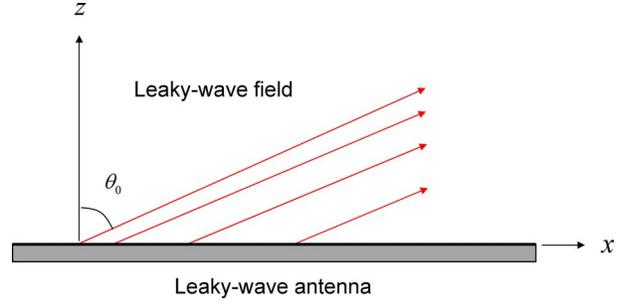
Figure 2b. The field of a leaky wave that is radiating from a leaky-wave antenna.
