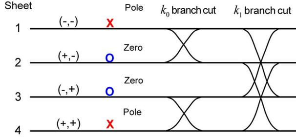
Figure 3. Side view of the Riemann surface, showing the four sheets along with the pole and zero locations on the different sheets.
