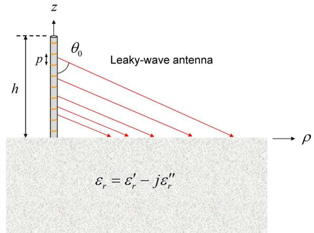
Figure 4. A vertical periodic LWA producing a near field that matches that of the Zenneck wave in a conical region (rotationally symmetric about the  $z$ -axis).
