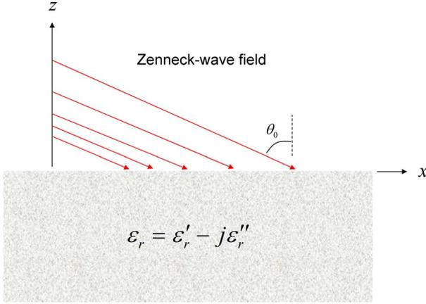
Figure 2a. The field of the Zenneck wave in the air region.
