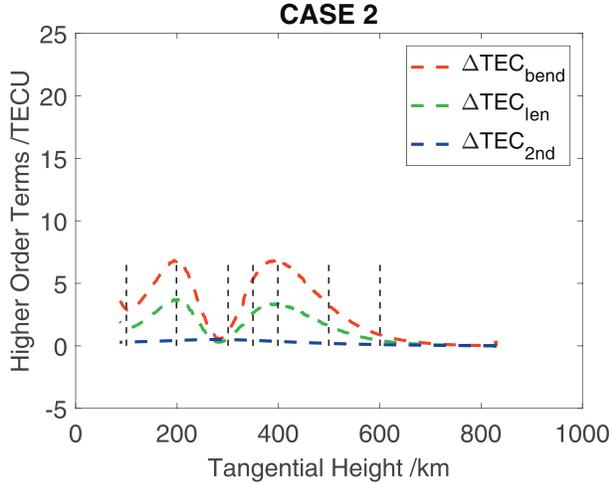
Figure 5. Variation of higher order ionospheric terms in RO TEC estimation as a function of tangential height for Case 2.
