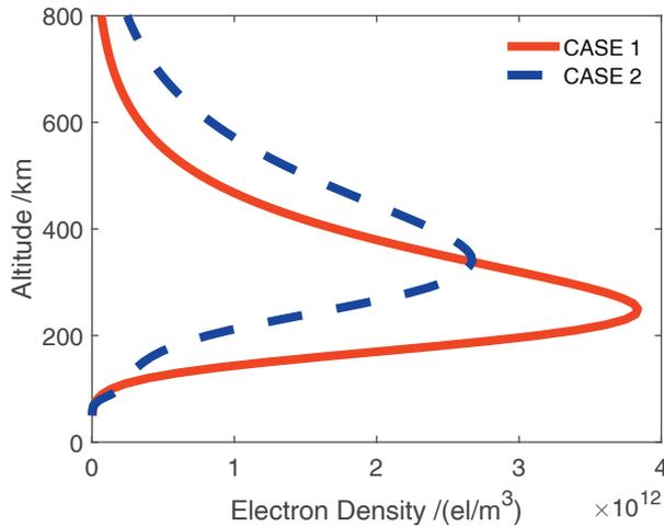
Figure 1. Case 1 and 2 electron density profiles generated by using three Chapman layers with vertical TEC (VTEC) = 100 TECU (1 TECU =  $10^{16}$  electron/m<sup>2</sup>). Case 2 was a thick profile (blue curve), with a relatively smaller peak density and larger scale height (profile thickness), whereas Case 1 was a thin profile, having higher peak density and smaller scale height.
