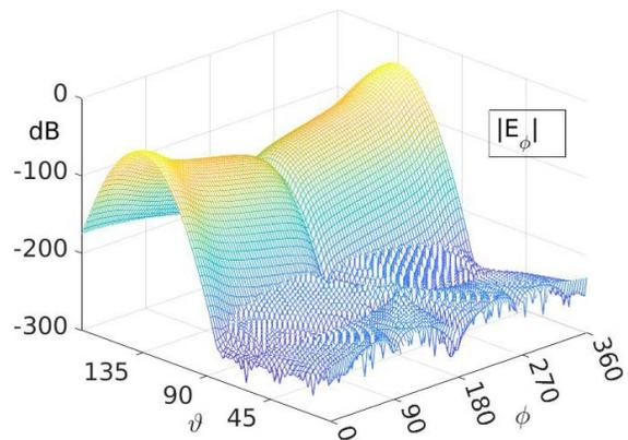
Figure 5. Normalized cross-polarized scattered far field of a UCSB magnetically polarized in the  $y$ -direction and incident on a half plane located in the  $xz$ -plane for  $x > 0$ . For the other data, see Figure 2.
