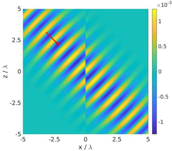
Figure 2. Normalized  $E_\varphi$ -component of a UCSB electrically polarized in the  $y$ -direction and incident on a half plane located in the  $xz$ -plane for  $x > 0$ . Waist at  $r' = 0.001\lambda$ ,  $\vartheta' = 45^\circ$ ,  $\varphi' = 180^\circ$ ; Rayleigh length:  $b = 10\lambda$ .
