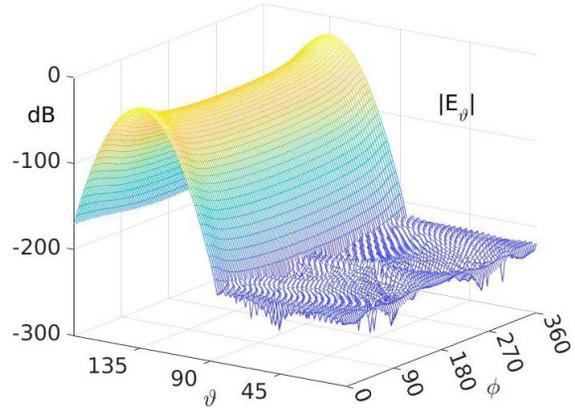
Figure 4. Normalized co-polarized scattered far field of a UCSB magnetically polarized in the  $y$ -direction and incident on a half plane located in the  $xz$ -plane for  $x > 0$ . For the other data, see Figure 2.
