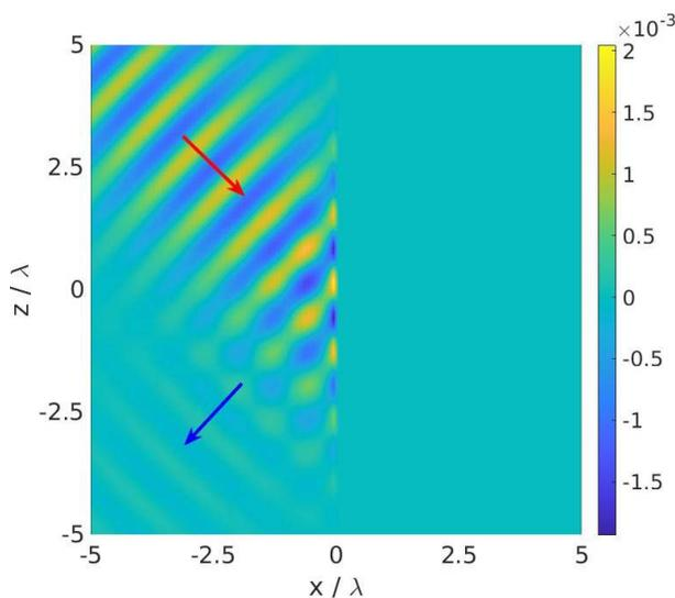
Figure 3. Normalized  $H_\varphi$ -component of a UCSB magnetically polarized in the  $y$ -direction and incident on a half plane located in the  $xz$ -plane for  $x > 0$ . For the other data, see Figure 2.
