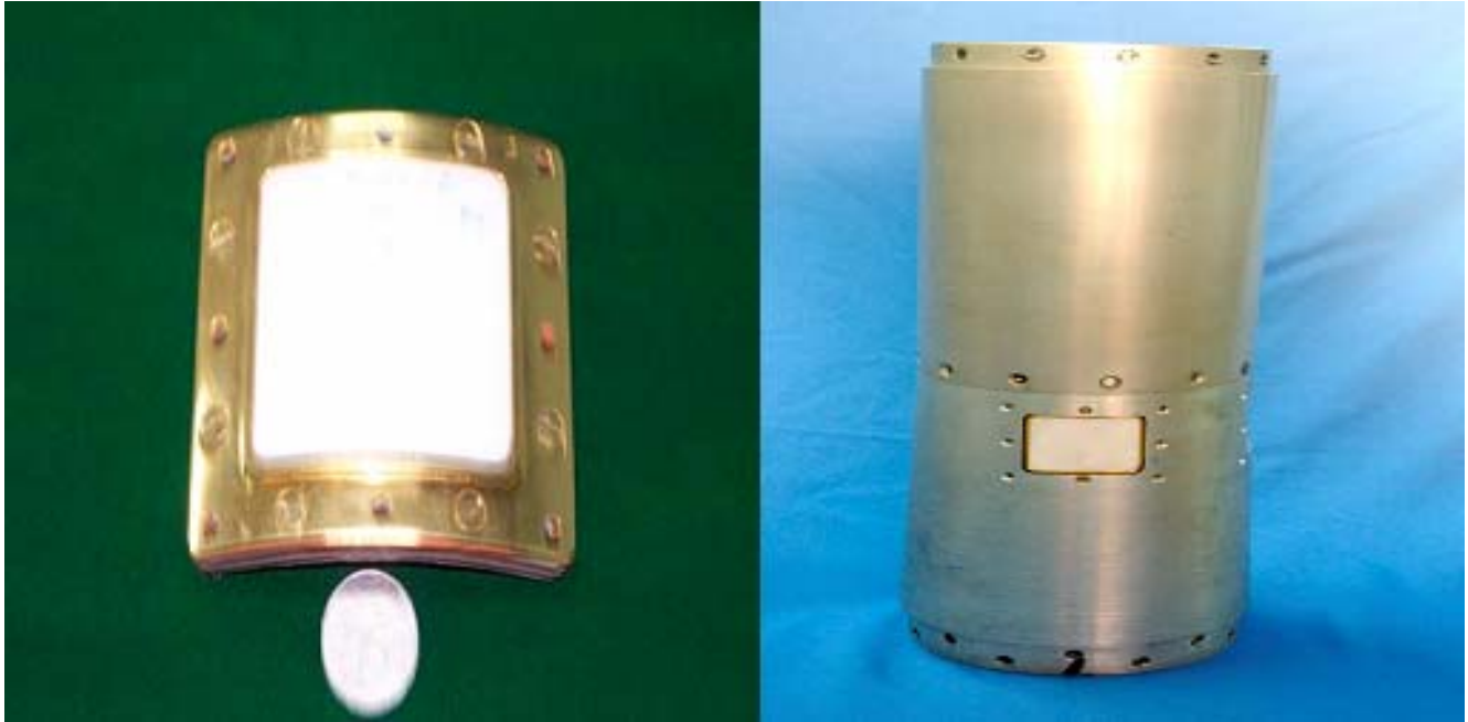
Fig. 1. Conformal Microstrip Antenna and mounting view.
