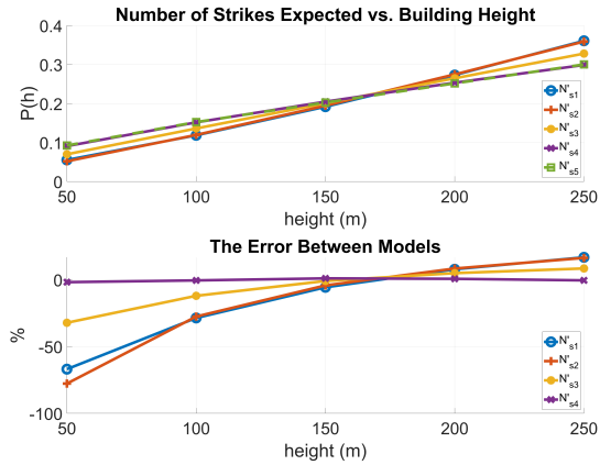
Figure 3. Top: The number of lightning strikes expected vs. height for three general equations, one case-study equation, and our model. Bottom: The percent between each equation and our model.
