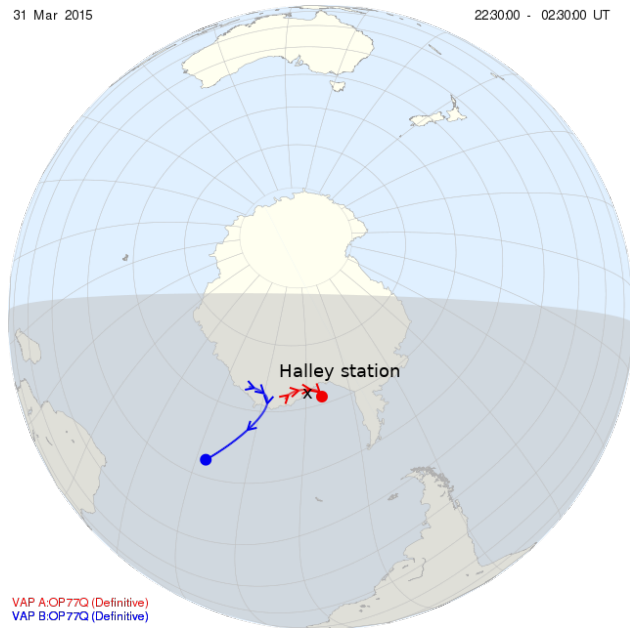
Figure 2: The magnetic footprints of VAP-A and -B close to Halley Station, Antarctica at 23:19:34.5 on 31 March 2015
