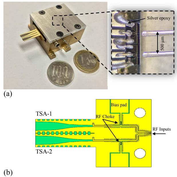
**Figure 1:** (a) A packaged photonic PAA emitter prototype with antenna and photodiode chips, inset: microscopic view of 2x1 UTC-PD array bonded to the antenna and (b) layout of the designed passive circuit board including 2x1 tapered slot antenna array.
