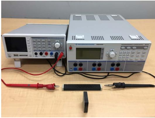
**Figure 2.** Photo of the measurement facilities including one power supply (R&S HMP4030) and one digital multimeter (R&S HMC8012).
