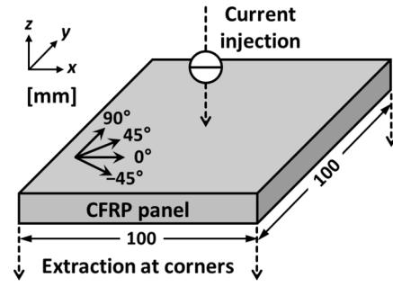
**Figure 6.** Lightning model for the 32-layer QI CFRP panel with the dimensions of  $100 \text{ mm} \times 100 \text{ mm} \times 64 \text{ mm}$ . Lightning current is injected at the center of the top surface and extracted at the four corners of the bottom surface.
