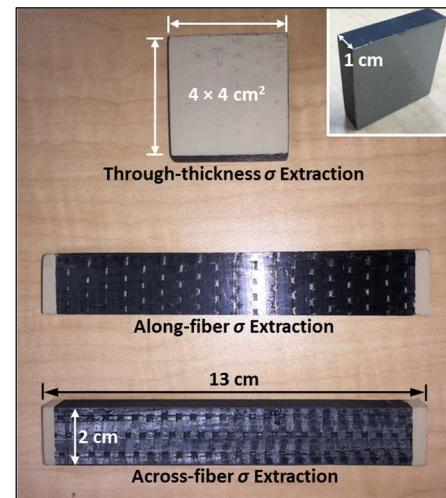
**Figure 1.** Photo showing the three CFRP samples for characterizing the electrical conductivity of three different directions. The samples were metalized with silver paste at their terminals.
