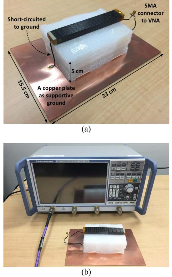
**Figure 3.** Photos showing (a) the setup of the AC measurement of a CFRP bar and (b) the measurement facility – vector network analyzer (R&S ZNB20).
