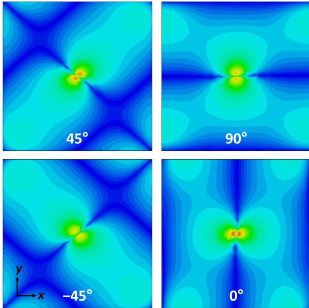
**Figure 7.** Distribution of current density of the top four layers of the 32-layer CFRP panel ( $45^\circ$ ,  $90^\circ$ ,  $-45^\circ$ , and  $0^\circ$  fiber orientations). The maximum magnitude denoted by red color is around  $2 \times 10^{11} \text{ A/m}^2$ .
