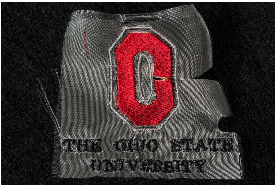
Figure 3. Colorful E-textile antennas fabricated via a hybrid approach that employs colorful threads on the front side and uni-color conductive threads on the back side.
