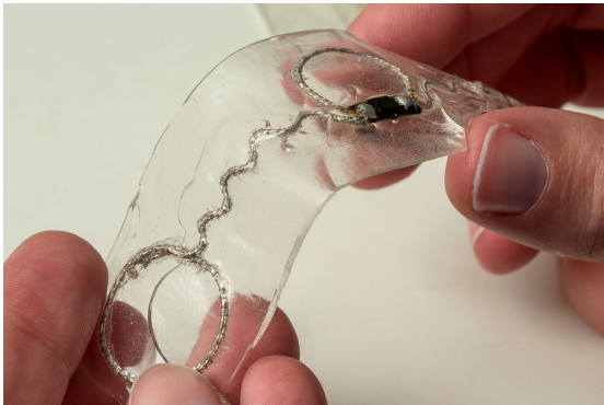
Figure 2. Stretchable and flexible RFID antenna fabricated by embedding the conductive E-thread into stretchy polymer.
