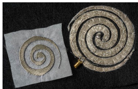
Figure 1. Flexible antennas fabricated via automated embroidery of conductive E-threads.
