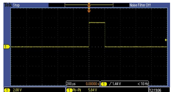
Fig. 5. Standard 1 PPS signal after transmission through Meinberg transducers and an optical fiber of approximately 300 m.
