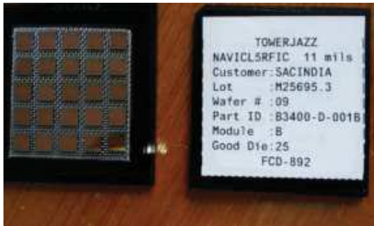
Fig.12 Fabricated dies in BiCMOS 180 nm Towerjazz process
