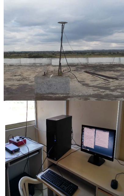
Figure 1. Septentrio PolaRxs-Pro GNSS receiver and antenna setup at GCET, Hyderabad
