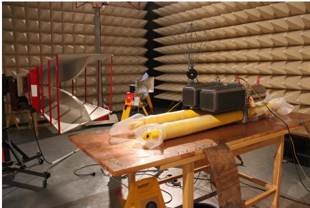
Figure 2. EMC measurements of the actuators in the anechoic chamber.
