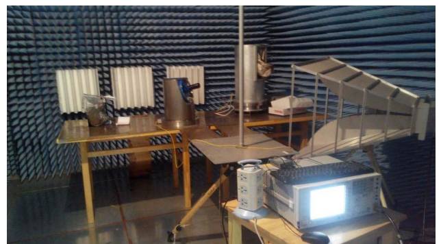
Figure 5. The SE measurements of one shielded cabin of the total station in the anechoic chamber
