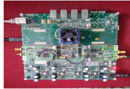
Figure 2 : WARP Xilinx Virtex-4 FPGA Board, popularly known as Mango Board
