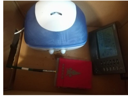
Figure 5. Experimental setup adopted for evaluating the sensitivity of the antenna performance to humidity.
