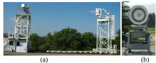
Fig. 4. Outdoor range measurement facility, (a) overview of the facility: left side is the tower for antenna under test in receiving mode, right side is the tower to install the Yagi-Uda antenna for transmitting signal, (b) the version-2 corrugated SBA under testing mounted on the outdoor near-field range measurement facility.
