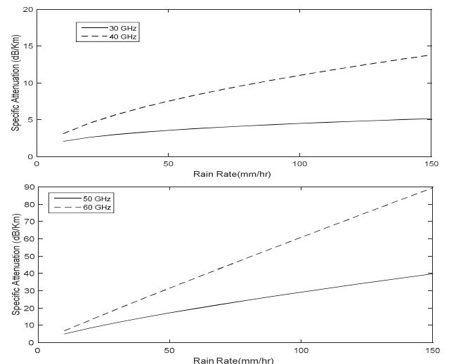
**Figure.1** Variation of specific attenuation against rain rate for different frequencies 30, 40, 50 and 60 GHz.
