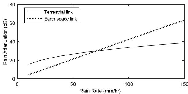
**Figure. 5** Plotting of rain attenuation as a function of rain rate for terrestrial link and earth space link of 5km path length at 30 GHz.
