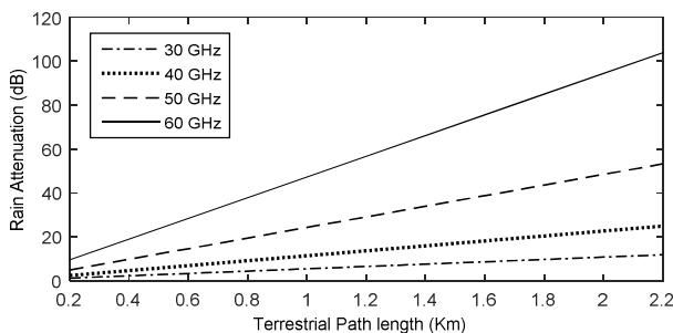
**Figure. 3** Plotting of rain attenuation as a function of terrestrial path length for different frequencies 30, 40, 50 and 60 GHz.
