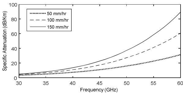
**Figure. 2** Variation of specific attenuation against frequency for different rain rates.
