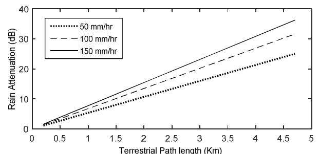
**Figure. 4** Plotting of rain attenuation as a function of terrestrial path length for different rain rates 50, 100 and 150 mm/hr.
