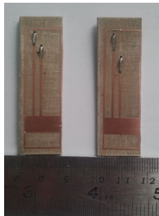
Figure 5. Photograph of fabricated multiresonator with two shorted stubs
