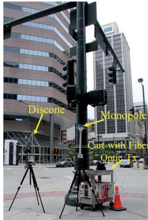
Figure 1b. A photograph of the two receiver antennas located at position R5, on the corner of Welton and 17th Streets.
