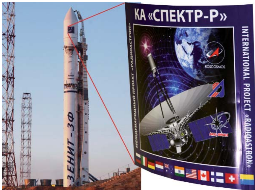
Figure 6. RadioAstron sitting on the Zenit rocket at the Baikonur launch site, ready for launch. The insert shows the imbedded plaque, displaying the international nature of RadioAstron.
