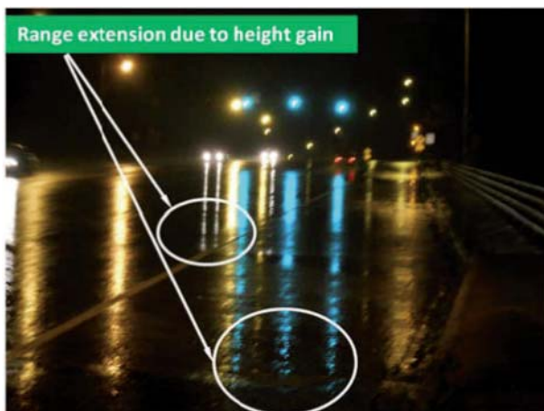
Figure 10. Waves on wet ground due to the partial reflectivity of the surface. The figure gives an impression of the physical propagation mechanism to be expected in cellular environments at frequencies where a wet Earth represents a complex impedance surface.
