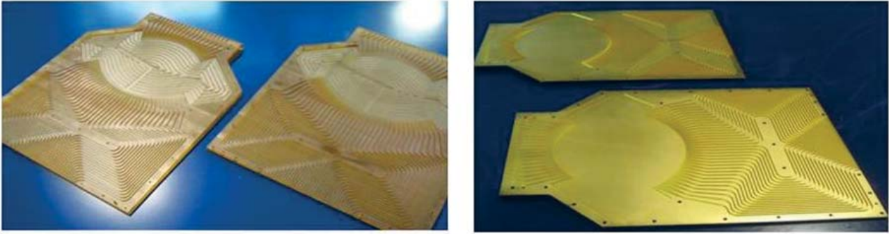
Figure 12. A Ka-band cavity Rotman lens made from Ultem 1000, and then gold plated.
