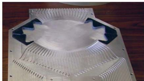
Figure 6. The second version of the Ka-band Rotman lens: integrated delay lines
