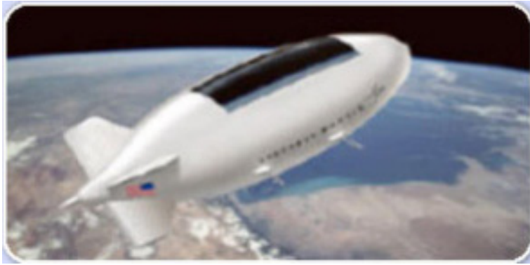
Figure 9 : An artist's impression of the Lockheed-Martin future high-altitude long-endurance HAP using a thin-film solar-cell array [21]
