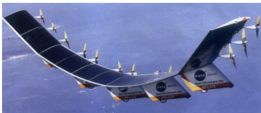
Figure 6. The Helios NASA experimental heavier-than-air solar-powered HAP flight over Hawaii, at an altitude of around 21 km in 2001 [15].
