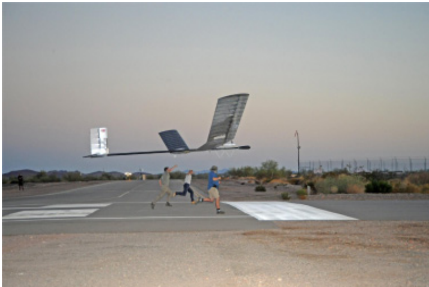
Figure 8. The launch of the QinetiQ ultra-light low-cost Zephyr high-altitude long-endurance UAV [22] (copyright QinetiQ).
