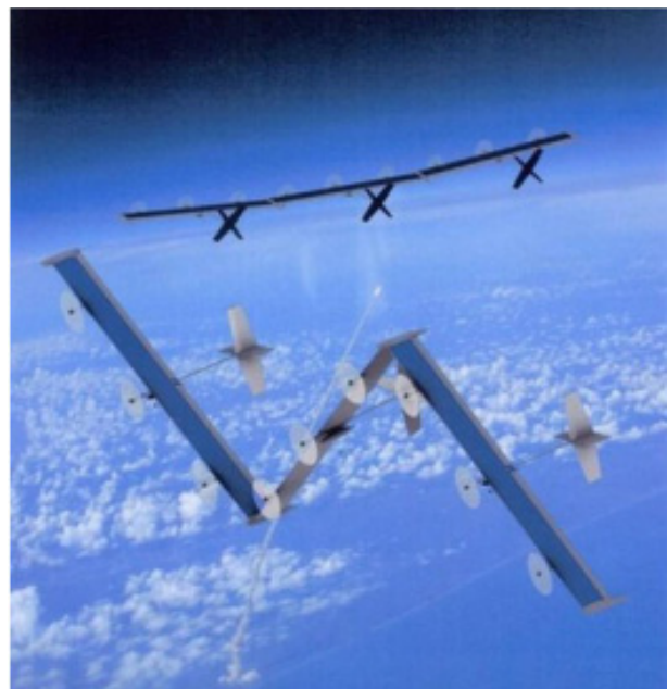
Figure 10. The Aurora Flight Sciences Corp. Odysseus future high-altitude long-endurance HAP concept. This is based on launching three separate planes and joining them together in the stratosphere [40].
