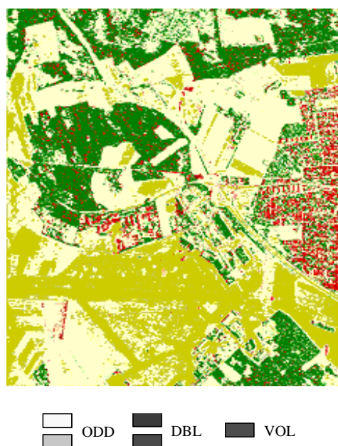
Figure 6. The selection of significant mechanisms and identification with canonical scattering mechanisms (ODD: single-bounce scattering; DBL: double-bounce scattering; VOL: volume diffusion).
