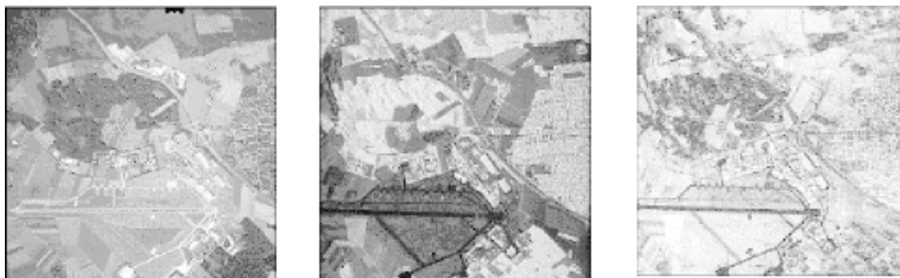
Figure 1. The optical image (left), polarimetric color-coded image (center), and interferometric coherence (right) over Oberpfaffenhofen (Germany).
