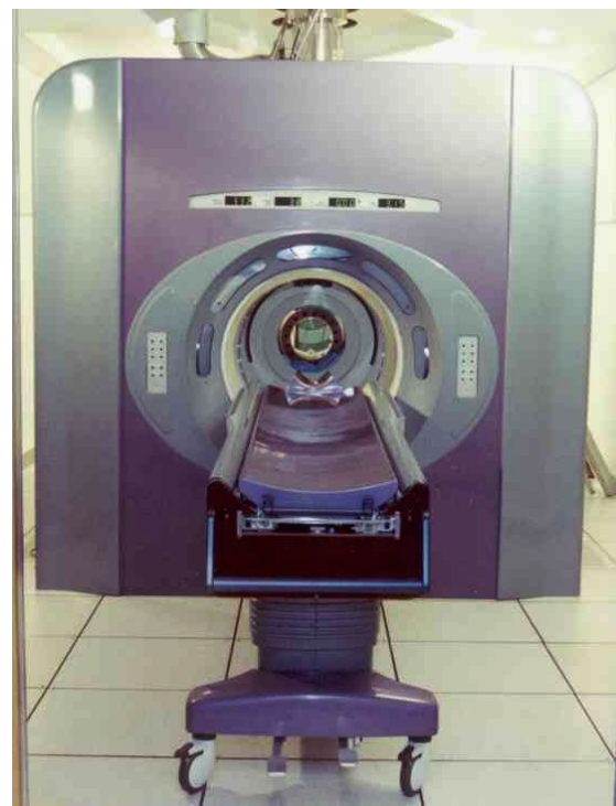
Figure 1. A view of the 8 T/80 cm human MRI scanner. The magnet is located within an iron room, built from more than 200 tons of iron, to contain the fringe field. The table is equipped with a cantilever top that delivers the subjects within the bore of the magnet. This picture shows the head gradient coil, the small cylinder at the center of the magnet.
