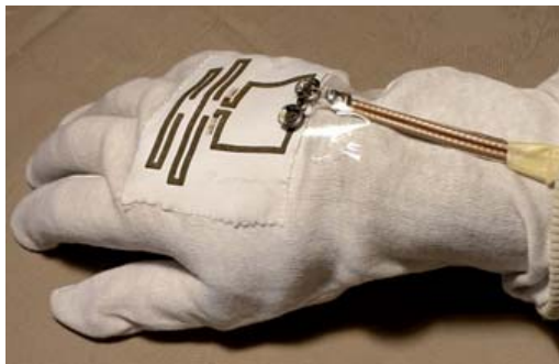
Figure 4c. A photo of a glove-integrated antenna worn on the hand.
