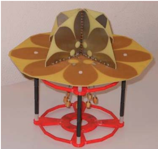
Figure 1a. A photograph of the Four Season vector antenna prototype (from [14]).
